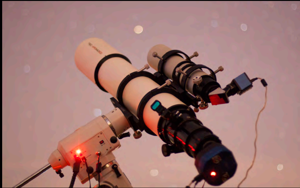
Modern amateur astrophotography setup using a cooled QSI CCD camera and computer guided mounting.
